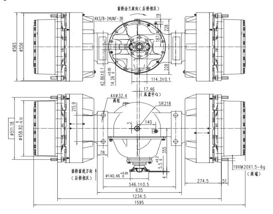
The Chinese-made CY20 axle can replace the American 14D axle, and all parts in the axle (except the axle housing and the main reduction part) are common
