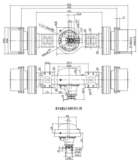
The Chinese-made CY40 axle can replace the German Kessler D101 axle, and the internal parts of the axle are common
