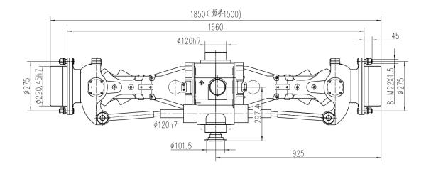
The 8T steering drive axle made in China can replace the American Dana 212 axle, and the internal parts of the axle are common
